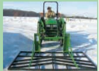
**MuSHGAL consists simply of a rectangular frame made from steel tubing.**
