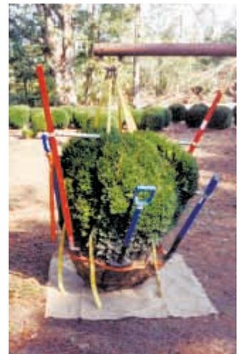
**Low-cost shrub mover uses a bunch of ordinary hand-held shovels held together by metal bars and nylon straps. It hangs from a 12-ft. “boom” that attaches to his loader tractor.**
