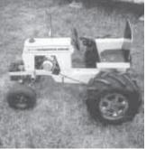
Minneapolis Moline pedal tractor (left) is powered by a Weedeater motor. Motorized pedal tractors can pull up to 1,600 lbs.
