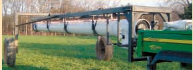
Feeder tows easily behind an ATV. Once on pasture, it's leveled-up and filled with 80 gal. of milk.
