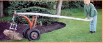
Manually-operated hand cart can be used to both lift and transport big rocks that
