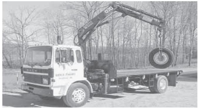
He uses this knuckle boom straight truck to pick up pallets, cultivators, even tractors.
