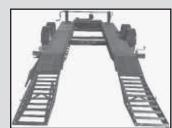
Trailer is loaded via a flip-up pair of loading ramps on back.
