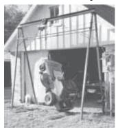
Electric-operated hoist allows Hussong to raise his Snapper riding mower. It measures 12 ft. high and wide, with legs spread 4 ft. apart.
