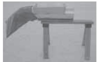
You put raw material into hopper and then tip unit up to fill bag.
