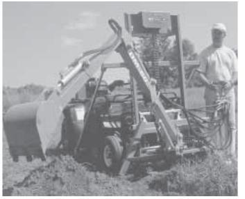
Backhoe arm has a reach of more than 7 ft. and can dig to a depth of 5 ft. It can be used to tamp and fill as well as to excavate.
