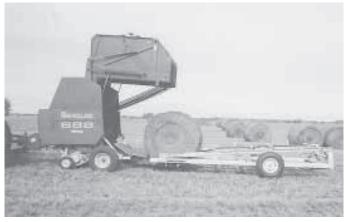
David Quick's Bale Buncher consists of a two-wheel trailer and a push plate hitch that bolts to baler axle.
