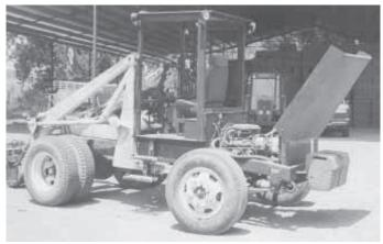
Troy Weyand converted an old 2 1/2-ton truck into this self-propelled bale handler.
