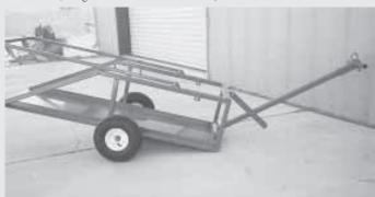
Cart has a metal floor and a hinged frame on top with a pair of hooks at one end.
