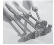
Branding irons have a 1/4-in. thick solid copper plate into which your design is machined. The copper plate attaches to a steel shaft with a wood handle.
