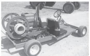
"When it fires it sounds almost like a shotgun going off," says Jack Deschene, who built this go-cart that's powered by an old 3 hp Deere E "hit and miss" gas engine.
