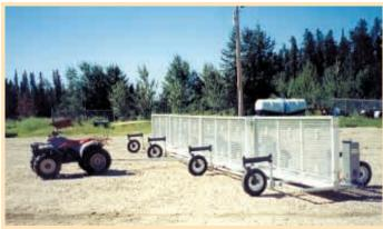
Field-size bug zapper consists of a 20-ft. wide by 4-ft. high steel mesh center panel, with a 10 by 4-ft. wing on each side. Each panel has three electrified grids.
