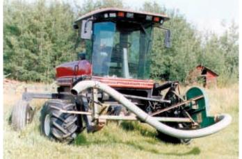
A section of steel hose taken from another old grain vac serves as the blower hose. He drove alongside canola swaths at 6 mph to blow snow off.
