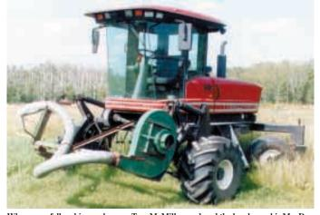
When snow fell on his canola crop, Tom McMillan replaced the header on his MacDon 2950 swather with the blower and pulleys off an auger-mounted grain vac attachment.
