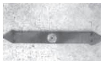
Holes were drilled at each end of bar to match holes in sickle sections, allowing him to bolt sections to bar.
