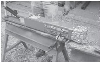
Mini "hand feed" replica baler produces bales that measure just 8 1/2 by 4 1/2 by 3 5/8 in. and weigh about 2 lbs.
