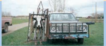
Chute mounts on passenger side of Dodge 1/2-ton 4-WD pickup. Both the headgate and swinging panel operate hydraulically.
