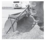
He used a 10-in. I-beam as the main frame and added a 3-pt. hitch and 3/16-in. thick plate steel for the sides. The blade is from a highway de partment snowplow.
