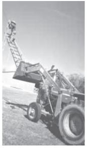
Ladder reaches 25 ft. up in the air. Prickett runs ropes from bucket to hydraulic controls on his tractor to raise or lower the bucket, so he can use the ladder when he's working alone.
