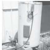
Electric scalder was made by modifying an old 50-gal, hot water heater.
