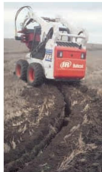
Trencher can be set at a steep vertical angle that allows it to turn sharply while digging. Augers pull dirt away from trench.
