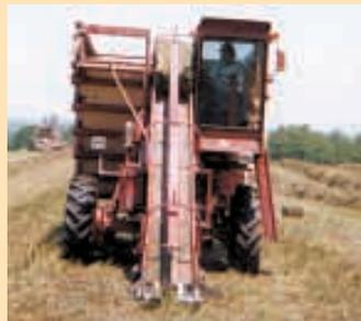
A grain elevator was converted to fit front of machine to pick up bales.
