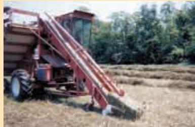
Arledge built bale hauler on the frame of an IH combine. Bale cage slopes to the back for easy unloading. When rear gate is opened, bales fall out all at once.
