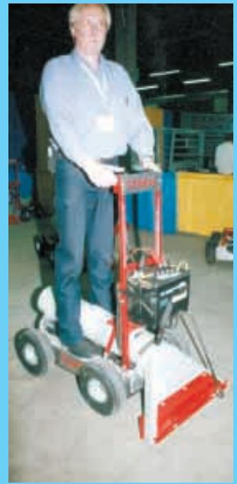
New 4-WD motorized nozzle cart supports a removable snout on front that hooks up to the hose on your grain vac. Operator uses hand controls to drive it around while standing on the unit. Eliminates the need to lift heavy grain vac hoses to clean grain out of a bin or quonset.
