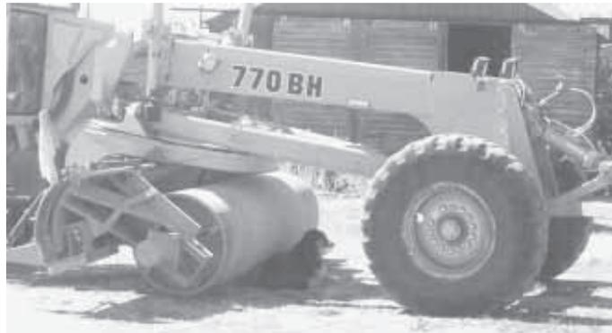
**Because roller is designed for easy attachment or detachment, grader operator can smooth new gravel or build a roadbed and then put on roller and compact his work.**
