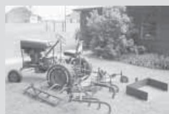
**Roy Lazenby Jr. built this garden tractor in the 1960's. "I made all kinds of equipment for it, including a 4-ft. floating finish mower, a garden cultivator, and a 3 by 4-ft. cargo carrier that mounts on the 3-pt.," he says.** mounts on the 3 pt. and turns it into a little pickup truck."
