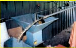
A branch cutter mounted on top of my tree chipper-shredder downsizes big branches to speed up the shredding process. The bolt-on bracket and branch cutter sells for \$70 plus S&H. (Dan Jacobson, 8913 Weaver Lake Dr., Pequot Lakes, Minn. 56472 ph 218 543-6623)
