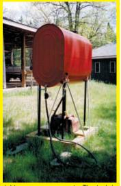
right on my own property. The tank is gravity fed and doesn't need a pump. It comes with a locking valve, fuel filter, 10ft. hose, swivel nozzle, gauge and storage platform. The entire unit can be moved on a snowmobile trailer. I'm willing to build units for \$575. (Dan Jacobson, 8913 Weaver Lake Dr., Pequot Lakes, Minn. 56472 ph 218 543-6623)
