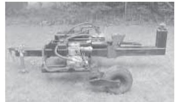
The same controls that operate the splitter are used to operate breaker bar.
