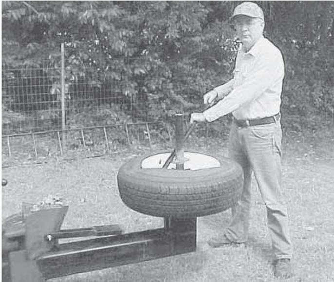
Jack Vines' wood splitter doubles as a tire repair machine, thanks to a set of removable attachments.
