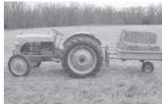
Trailer's single caster wheel pivots 360°, letting Marks back up just like backing a car.
