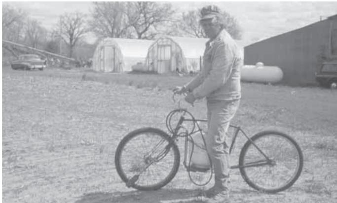
Reynolds stretched bike frame to carry propane tank and mounted burner nozzle on front wheel.
