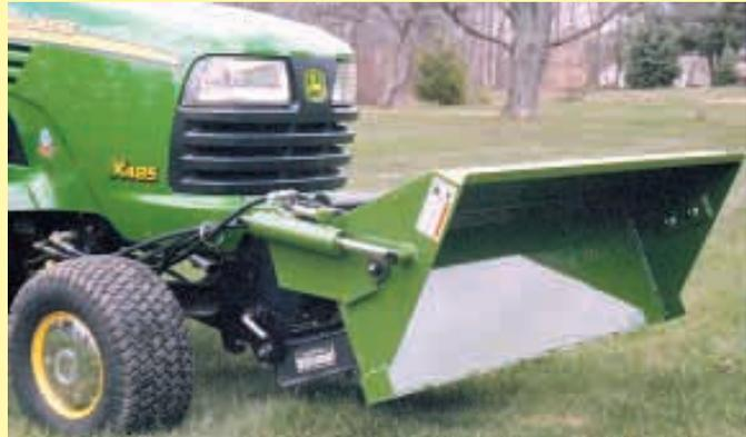
Bucket carries 2 1/2 cu. ft. of material. It fits on front hitch of Deere 425, 445, 455 and new X models.
