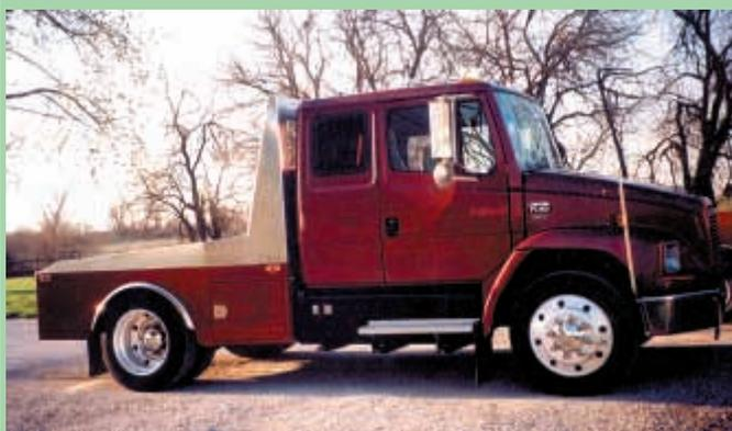
Freightliner cab has bunk behind front seats, a 120-decibel horn on top, and a "western hauler" bed on back fitted with a gooseneck ball.
