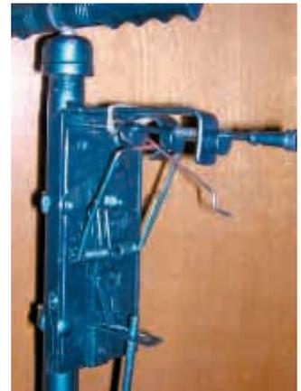
Top handle on trap is raised, left, to cock sharpened spear inside 3/4-in. dia. pipe. Rat trap, right, connects to trigger that runs down to bottom of trap. When mole activates trigger, rat trap instantly releases spring-loaded spear.
