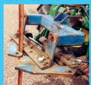
Post puller consists of a steel jaw that's hinged in middle and is attached to a hydraulic cylinder. Extending the cylinder closes jaw around post.
