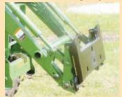
Steel mounting plate accepts skid steer attachments like posthole augers, left. Photo on right shows closeup of mounting plate on loader.
