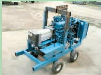
Belt-driven generator powers an electric motor, which operates a pressure pump that delivers water to handheld spray wand.
