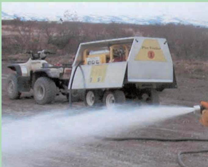
Fire fighting equipment is contained in two metal trailers that can be pulled behind pickups, ATV's, or even snowmobiles.
