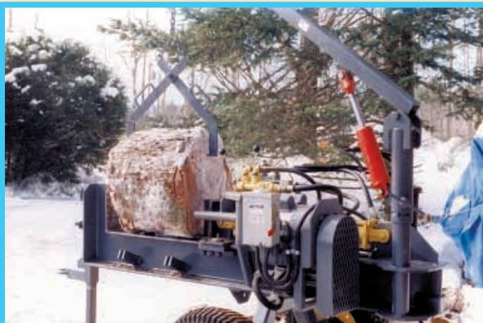
Wood splitter is powered by a 240-volt, 3 hp electric motor that belt-drives a hydraulic pump.
