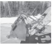
Fold-up forks pin to a pair of brackets welded to each side of loader bucket. Forks can be quickly flipped up to use bucket for other work.
