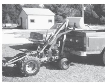
Hartman uses a hand-cranked boat winch to raise and lower loader, and a long trip handle to dump the bucket.
