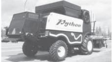
Rite Way's new combine replaced 75 percent of the belts and pulleys found on most combines with hydraulic motors.
