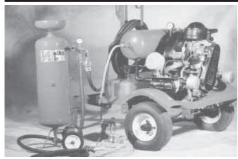
Air compressor kit turns VW engine into high capacity sandblaster.
