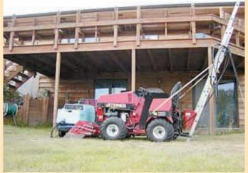
To attach ladder, Bergman ran a steel rod through bottom rung and then through the lift arms on tractor 3-pt. Then he ran two support straps up to a rung about halfway up
