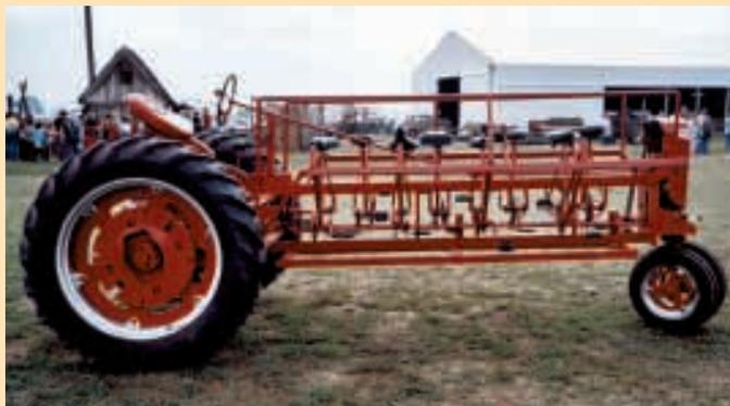
Rubison removed the engine and mounted two banks of four bicycles back to back. He says just one person pedaling can move the tractor.
