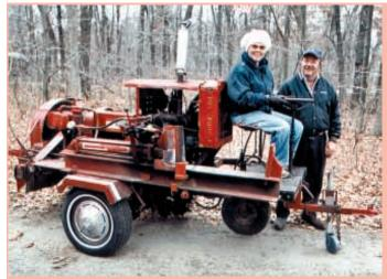
Gerald Krob converted his wood splitter to this self-propelled model that's also equipped with a 32-in. buzz saw.
