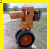
I unbolted the front end of the tractor and bolted on a fake radiator that I made from steel plating. The mailbox itself is a short length of 10-in. dia. auger tube. After making a door for the mailbox, I welded a bracket on back of the grill to hold a flower basket. The tractor mounts on a length of 3 1/2-in. sq. tubing anchored in cement 5 ft. underground. (Allen and Cindy Clow, 3739 230<sup>th</sup> Ave., Lancaster, Minn. 56735)
