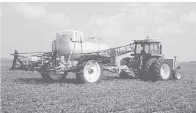
Sprayer is equipped with a 1,600-gal. tank and 80-ft. boom. “It works great for applying post-emergence herbicides in corn and beans,” says Olson.
