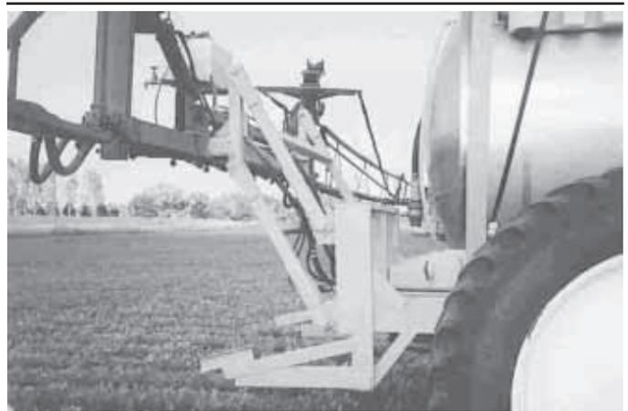
To hold the boom, they added a hydraulic parallel linkage constructed from the wings of an old Wil-Rich cultivator.
