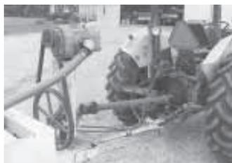
Air compressor mounts on trailer hitch and is pto-driven off tractor.
