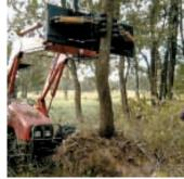
Tree is rocked back and forth to loosen the roots before it is pulled out.
