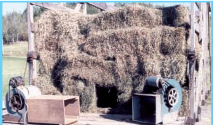
**Wooden box on fans directs all air into stacked bales, drying them in a couple days without any source of artificial heat.**
