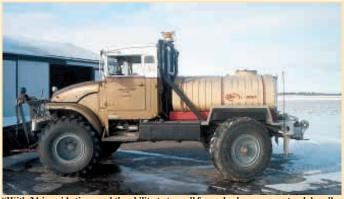
"With 24-in. wide tires, and the ability to turn all four wheels, my spray truck handles especially well on steep embankments," says Harry Engeland.
