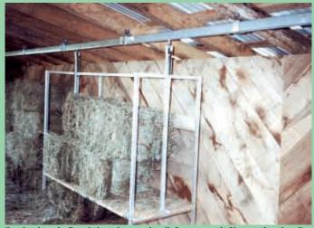
Overhead track allows bales to be moved easily from one end of barn to the other. One shove is all it takes to move carrier the length of barn.
