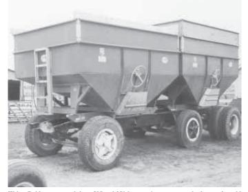
Walter Baldner mounted these 525 and 250-bu. gravity wagons on the frame of an old tandem axle truck. "By pulling a 350-bu. wagon behind the two boxes, I can haul about 1,100 bu. at a time," says Baldner
