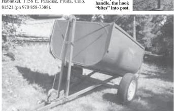
Two-wheeled, pull-type dump trailer was built out of a 265-gal. fuel oil tank and a boat winch that mounts on the tongue. To dump the load, Prom simply cranks the winch.
