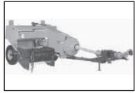
Mini round baler, left, makes bales that measure 20 by 28 in. and weigh just 40 to 50 lbs. Mini square baler, right, is designed specifically for 15 to 20 hp tractors.
