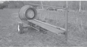
As tree leaves cone, it drops onto a wooden platform that extends the length of the machine.
