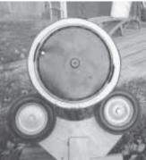
Lawn mower wheels hold drum to allow it to rotate freely.
