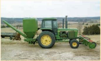
Harry Thompson's tractor-mounted "stripper" harvester is designed to strip seed from any standing loose-headed grass or small grain crop.
