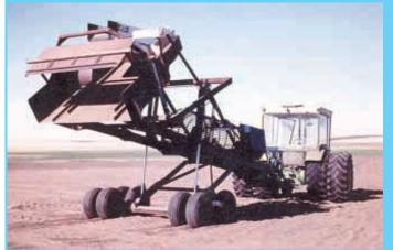
Clifford and Clarence Arnal enlarged the hopper on their Harley rock picker and designed a new scissors-type lift to dump hopper into truck.
