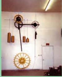
One entire wall of Harry Benjamin's shop is taken up by a giant 16-ft. pendulum clock he made out of old farm machinery parts.
