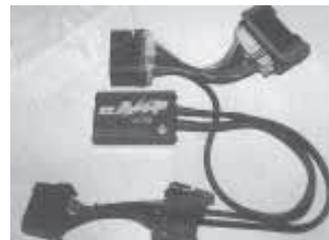
Plug-in chip reprograms engine's computer to alter time and duration of fuel injection according to load.
