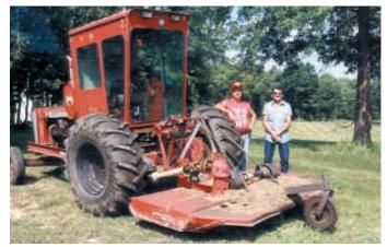
Bob and Rick Smith built this self-propelled mower out of parts from an IHC 403 combine and an Oliver 1850 tractor. A Bush Hog 10-ft. mower deck mounts on front.
