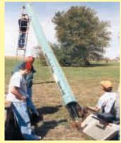
Pumpkin launcher works something like a sling shot, using a 20-ft. length of PVC pipe as a barrel. Exercise bike pulls pumpkin down for launching.
